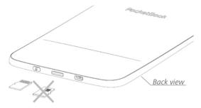
To eject the card, slightly press on its edge until it will be unfixed, and pull it to get.
